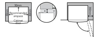
If you have a cupboard above the refrigerator with a rear gap of less than 100 mm (Y), recommended clearance at the top of the refrigerator increases from 50mm to 90mm (X) minimum.
